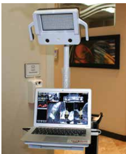
Fig. 1_ The Navident system is shown here with the Micron Tracker and laptop loaded with the Navident software.
