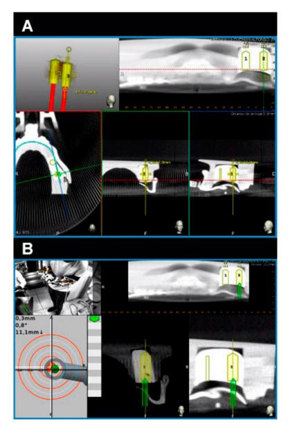
**Figure 2.** (**A**) Dental implant planning as seen in the treatment-planning software of the computeraided dynamic navigation system (yellow cylinders) and (**B**) dental implant placement (green cylinders) controlled at all planes and depths.
