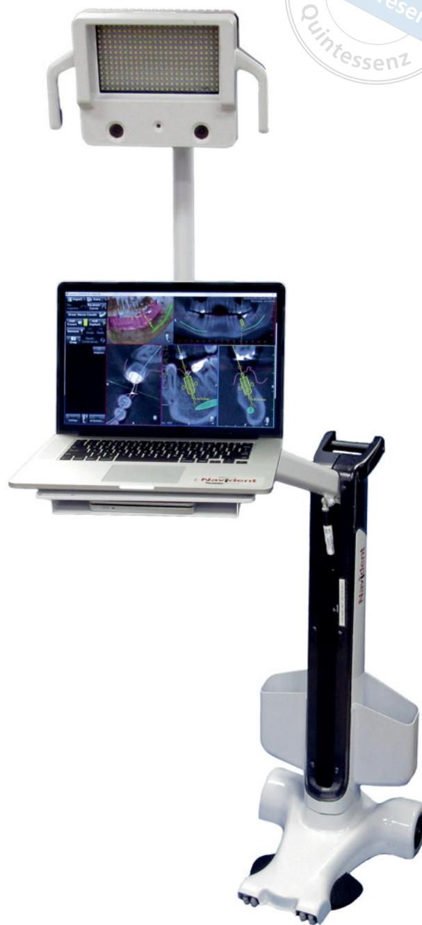
Fig 1 The Navident (ClaroNav) mobile unit with an overhead light, stereoscopic motion-tracking cameras and a mounted laptop computer with uploaded implant planning software.
