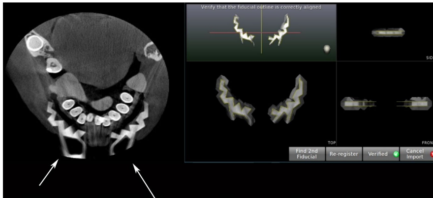
FIGURE 3 Automatic registration using fiduciary markers/tags (arrows)
