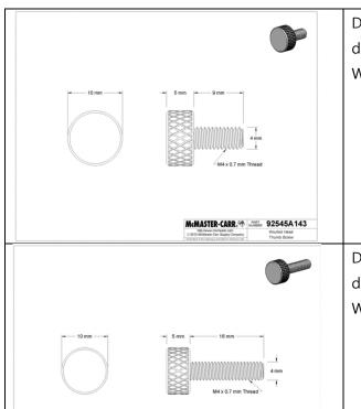
Dimension: 9mm long thread, 10mm head diameter, 5 mm head height.
